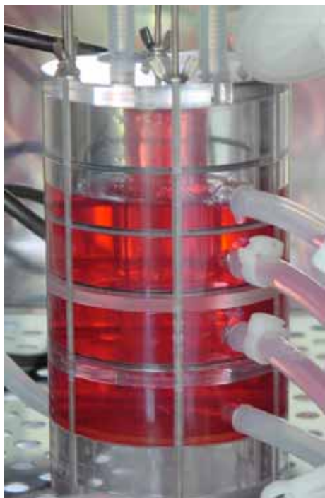
Figure 4. "Bioreactor" system developed by the Jockenhoevel group for mechanical conditioning of autologous heart valves prior to implantation.
